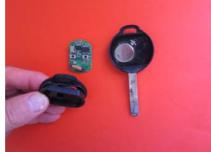
2. Remove old rubber key button pad from plastic key button insert.
