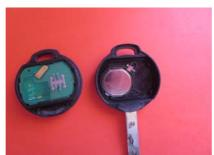
1. Prise open your remote with small screwdriver to end up with 2 main shell parts:
